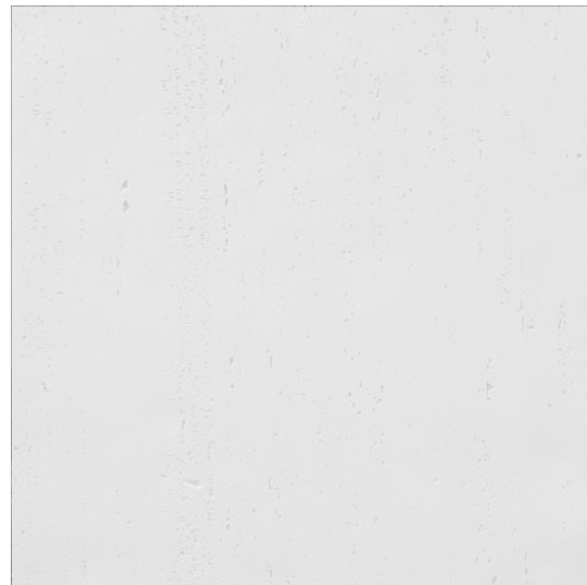
PCP.2 PRECAST CONCRETE WALL PANEL EXAMPLE SMOOTH FINISH WITH WHITE NAWKAW STAIN
