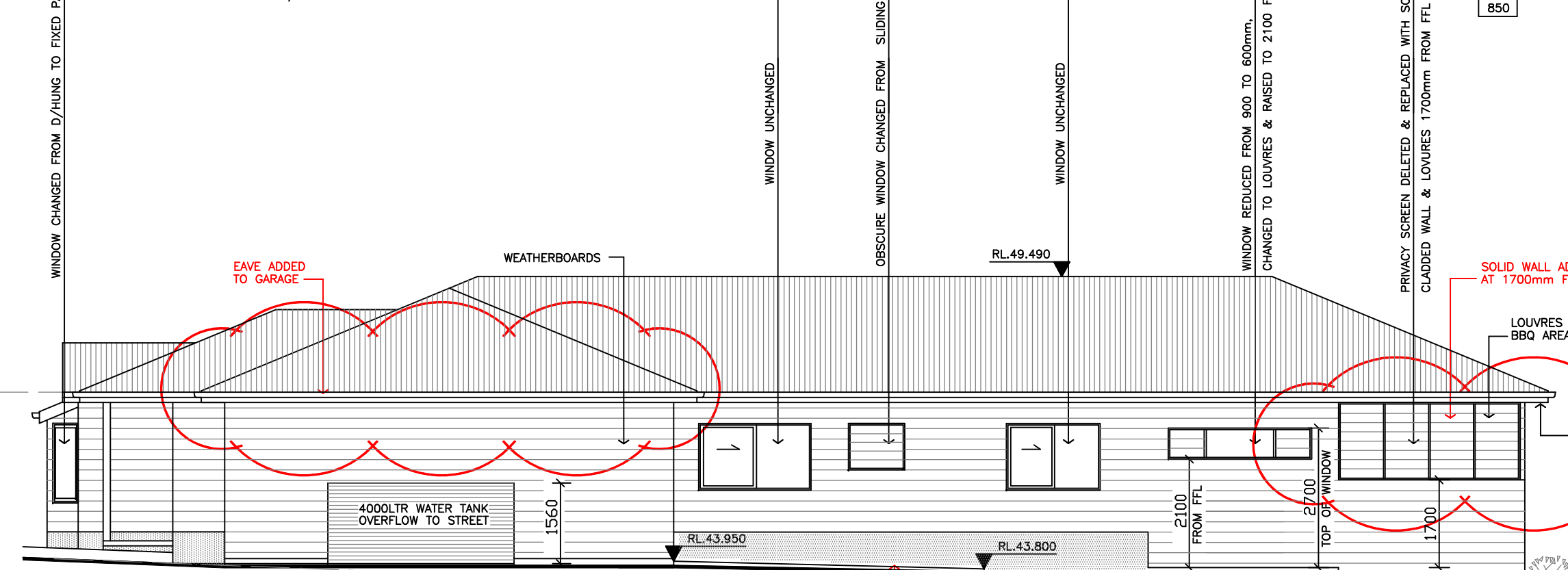
WESTERN ELEVATION PROPOSED/UNDER CONSTRUCTION
