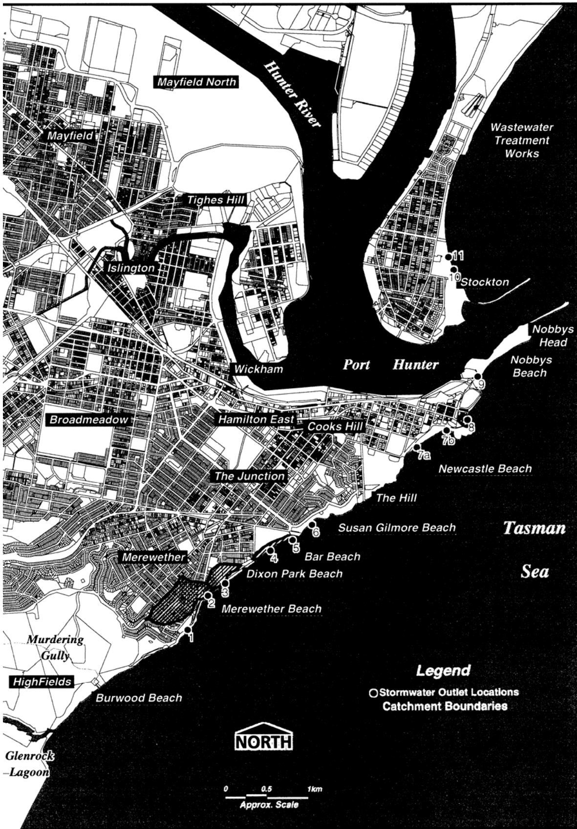
Figure 13: Coastal Zone Stormwater Outlet Locations
