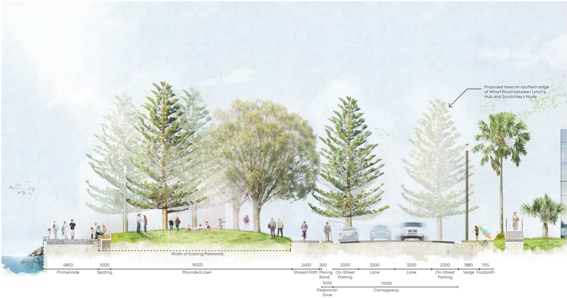
Foreshore Typical Condition (Section A-A) (TCL, 2021)
