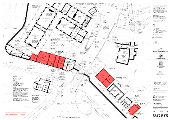
Figure 42. Floor plans showing WWII additions. A new guardhouse and generator room were constructed to the east of the gates. The Old Guardhouse was extended to the west and a new rations block was constructed between the NCOs' Ablutions and the Old Guardhouse. Internally, a new wall was inserted in the Old Guardhouse separating the southern cell from the main room. (Source: Gate/Courtyard Floor Plans Lower, 2005, Suters Architects)
