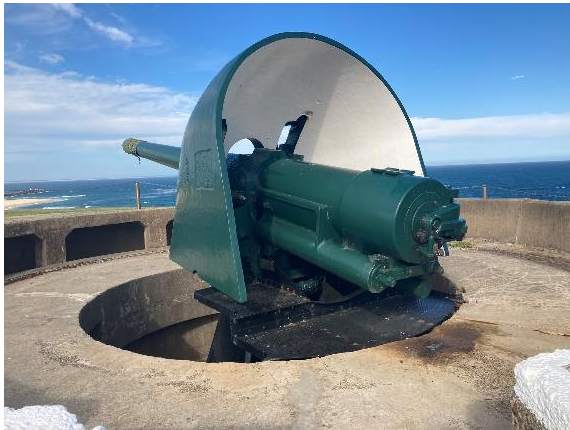
Figure 193. View of No. 1 Gun, one of a pair of 6 inch Mk VII BL guns. (Source: CPH, 2023)
