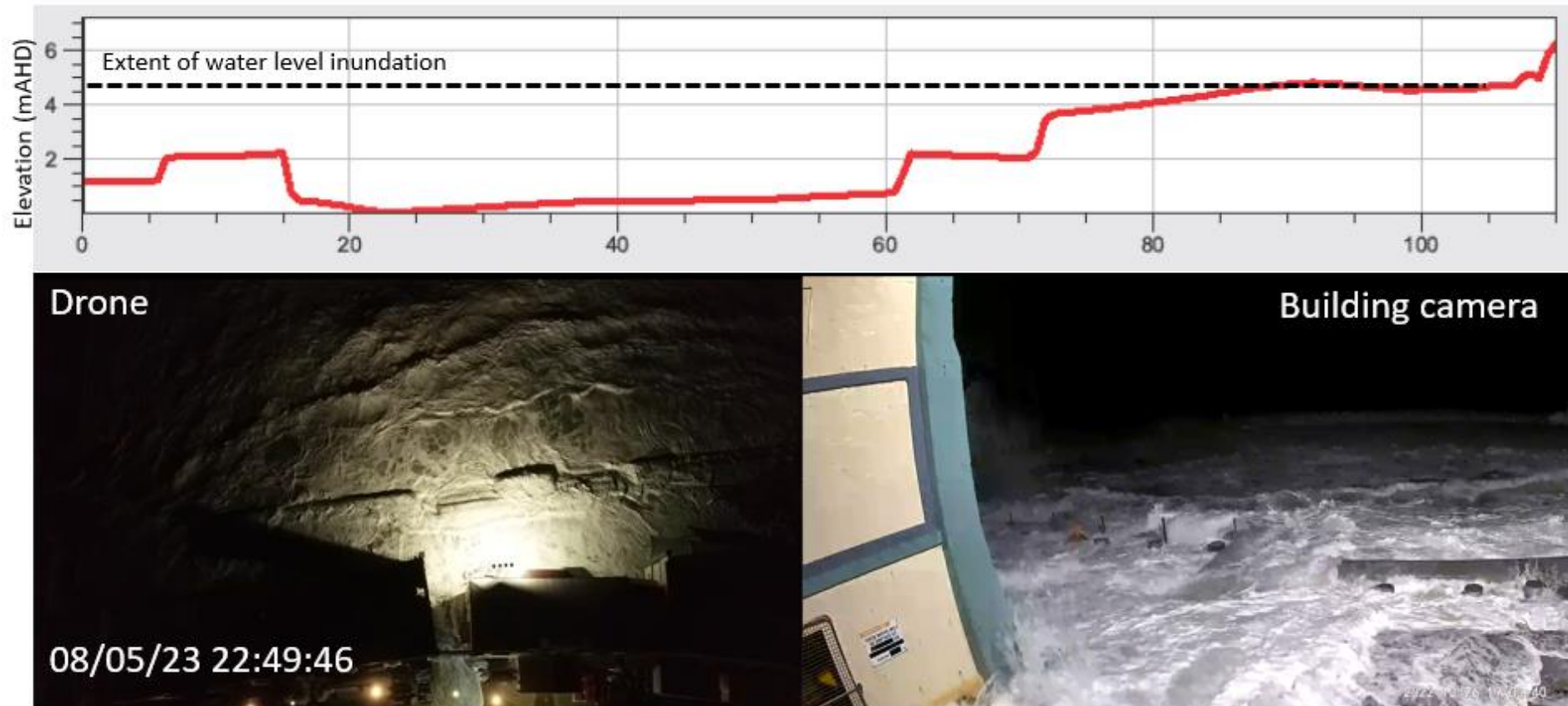
Figure 61: Observed inundation level derived from the drone marked against the digital elevation model for the pre-works facility.
