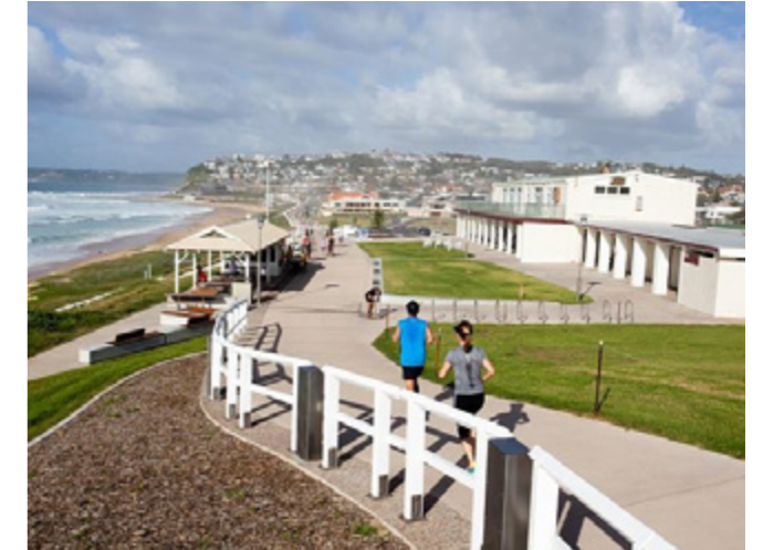
Fencing along the Newcastle Bathers way coastal walk, made from recycled wood and plastic materials
