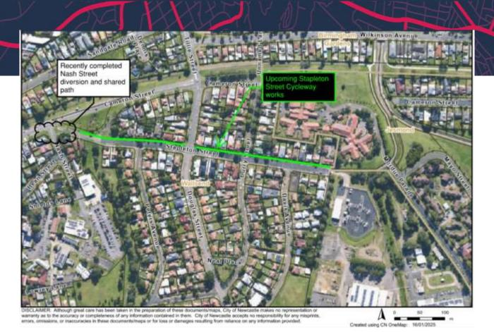
These works provide an on road bi-directional cycleway between existing the kerb and gutter and proposed offset parking lane. It provides for two parking lanes and narrower travel lanes and retains existing footpaths for pedestrians.
